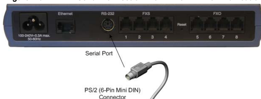
Figure 2-6: MP-11x Serial Connection with PC for CLI Communication
